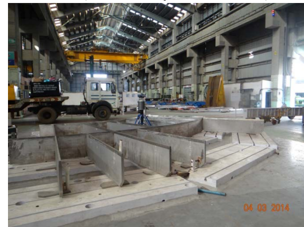
Manufacture of VV Sector#6 and lower port inner shells (courtesy of KO DA)
