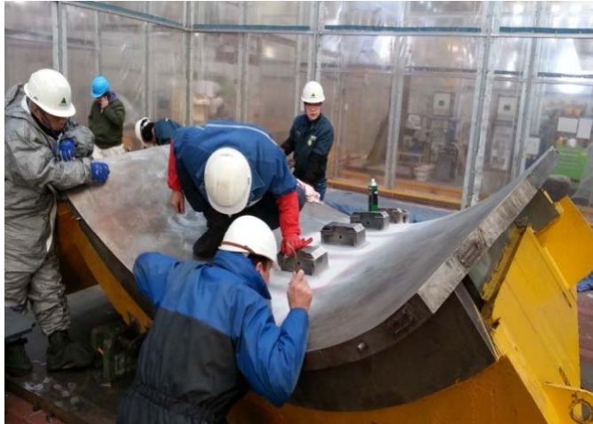
Manufacture of VV Sector#6 and lower port inner shells (courtesy of KO DA)
