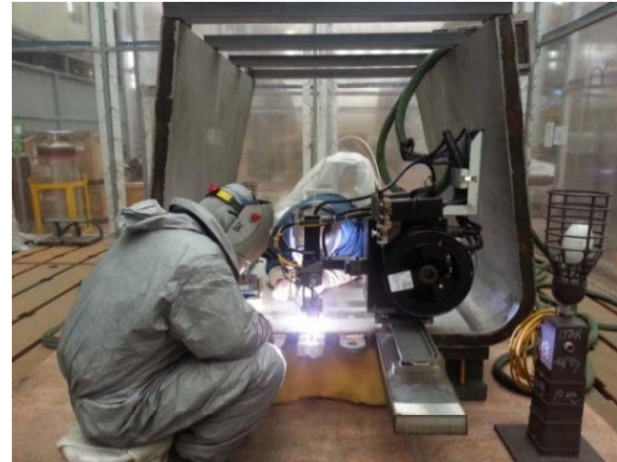
Manufacture of VV Sector#6 and lower port inner shells (courtesy of KO DA)
