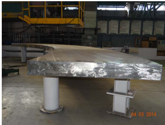
Manufacture of VV Sector#6 and lower port inner shells (courtesy of KO DA)
